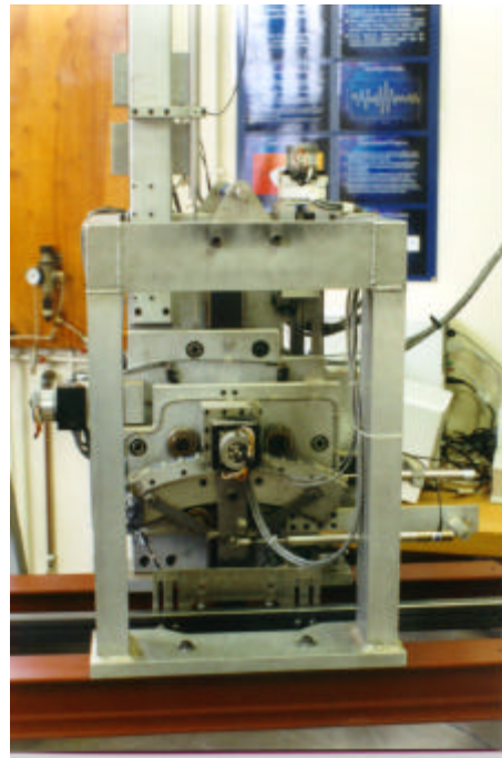
Figure 1 - Photograph of the three degree of freedom loading rig located at The University of Oxford.
