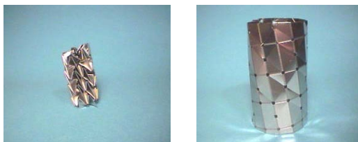
An origami stent made from stain-less steel. Its diameter expands from 12 mm to 23 mm.
