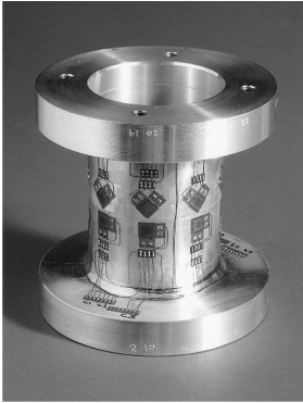
Figure 6. The 6 degree-of-freedom load cell.
