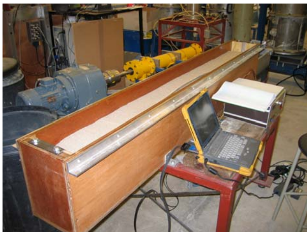
Figure 9 : Set-up for small scale 3-D buckling tests.
